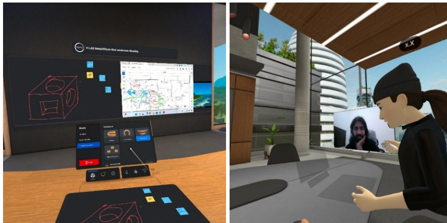
Fig. 6. Model modification and interdisciplinary discussion. (a) Overlay of suggested design changes within the shared BIM model. (b) Group interaction and debate on multiple design items across VR and desktop interfaces.
